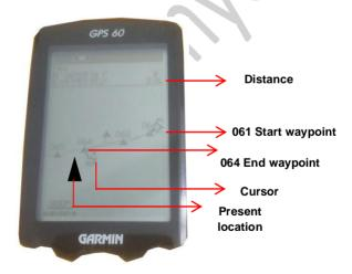
Note: In advance GPS set, to measure distance from current location, press "Page" button to open "Map page". The present location cursor, waypoints and tracks appear on the screen, press "Menu" once, and select "Measure Distance" option from the list and press "Enter". Using "Rocker Key" move your cursor arrow from the current location (Shown in Black triangle). While moving the cursor, a line with distance in Km will appear.
