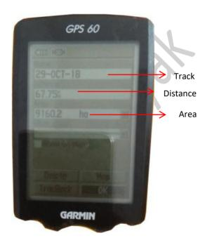
Note: In advance GPS set, to measure area calculation, Press "Menu" button twice and scroll down with "Rocker Key", select "Area Calculation" and press "Enter". Press "Start" and walk around the area to be measure. When reach on end location, press "Calculate" option with "Enter" key. Area in units will appear on the screen. Units can be change under "Change Units" option and select "Save track".
